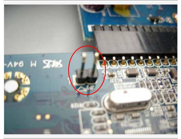
4. Connect the two jumps(pins) to form a short circuit. Then plug in the power and hold the short circuit for more than 10 seconds.
